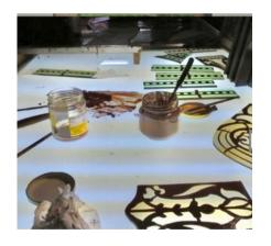
Then, each section was laid out on a table and new caming (lead) was placed between each small piece, and the entire panel was then bonded.
